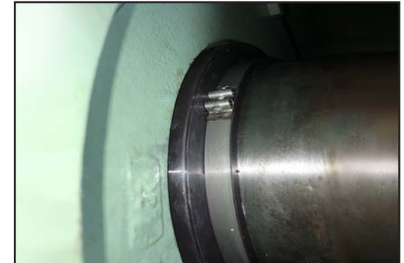
Split Polymer Labyrinth Seal installed.
